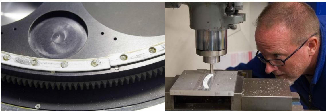
Figure 20 – Left: Image showing some of the damaged sapphire balls in the lower filter wheel prior to removal. Right: Careful machining of new Teflon spacers.
