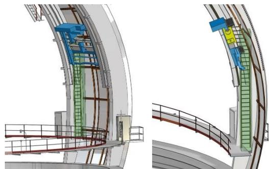
Figure 24 – Bridge crane access conceptual designs.
