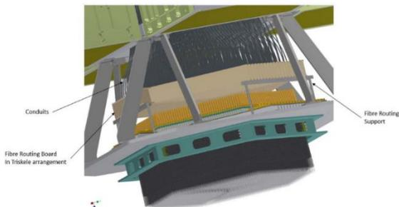
Figure 78: Fiber routing within the Fiber Positioner
