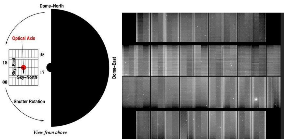
Figure 16 - Left: Schematic of MegaCam shutter. Right: MegaCam Exposure binned by a factor of 24 to illustrate the occasional noise patterns visible on CCDs in the second row.
