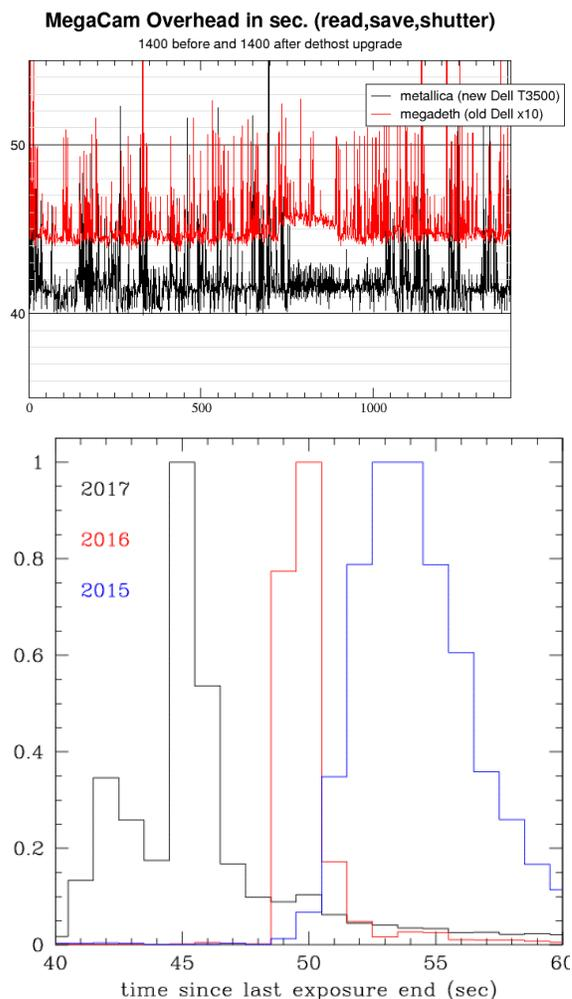
Figure 15 – Top: The x-axis shows the number of exposures tested and the y-axis gives the total overhead time before (red) and after (black) upgrades, including reading, saving and shuttering. Bottom: Histograms (as of Sept 18, 2017) of dead time between all exposures archived at CADC during 2015 (blue), 2016 (red) and 2017 (black). Figure courtesy S. Gwyn.
