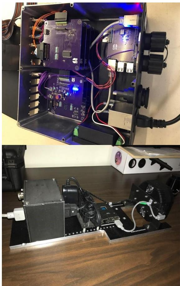
Figure 23 – Top: TCS RBUSS replacement hardware is shown. Bottom: New TCS Cassegrain CCD guide camera and mount, ready to be deployed on the summit, is shown.
