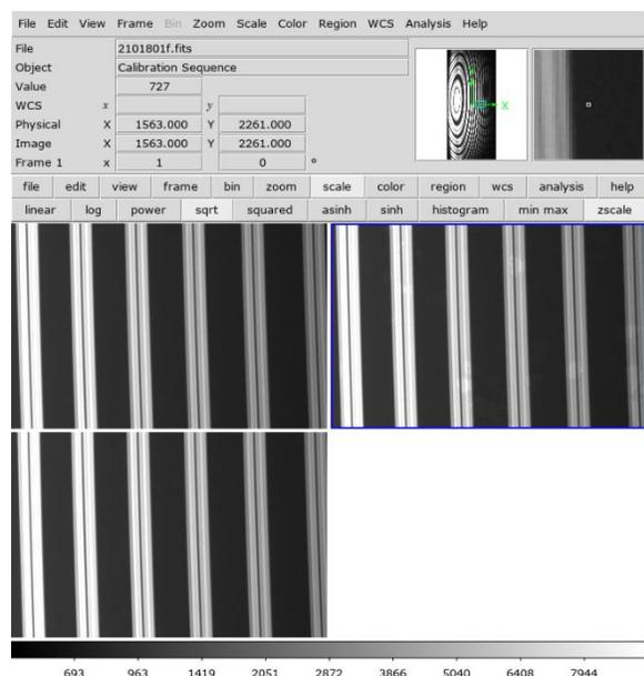
Figure 21 - ESPaDOnS flat-field images from before (upper left), during (upper right), and after (lower left) the "splotches" were visible.
