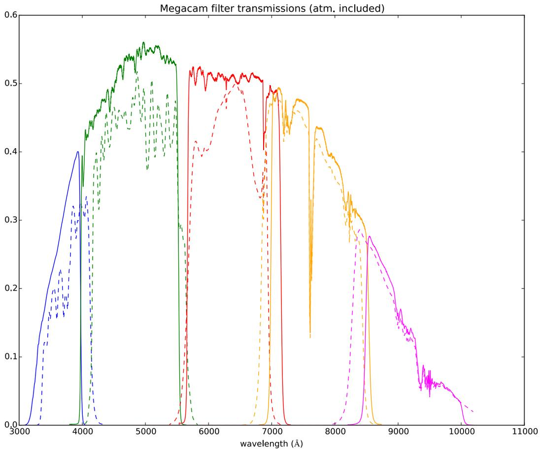
Figure 2. Full transmission spectra in the old (dashed lines) and new (solid lines) broad Megacam bands, including the filter transmission themselves, as well as the transmission of the different parts of the Megacam optics (wide field corrector, lenses), the telescope primary mirror, and an average atmospheric transmission above Maunakea at an airmass of 1.25 (see Betoule et al. 2013, Buton et al. 2013).
