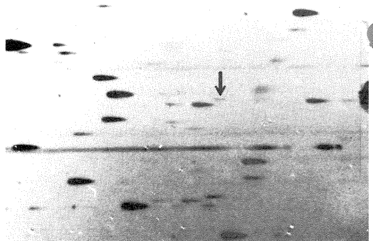
Green grens spectra of the field pulsar 3C 36 (see arrow) taken with the valve electronographic camera mounted on the wide field corrector. The quasar is as faint as magnitude B=22.3 . Despite this, it was obtained with the grens in two hours exposure on Ilford L 4 emulsion, with a high signal-to-noise ratio.
