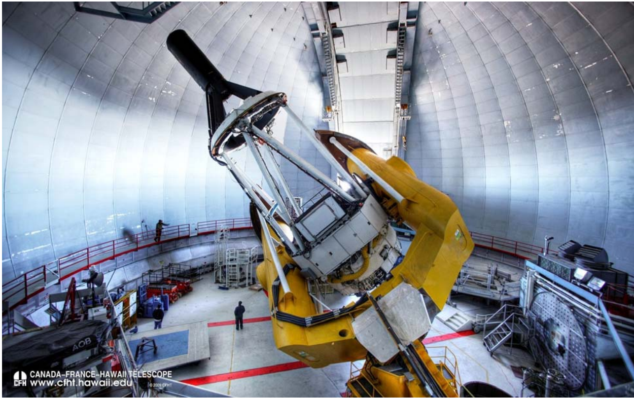
CFHT dome interior. The inner catwalk is seen with red handrails. Power slip rings are enclosed by screening below the inner catwalk.
