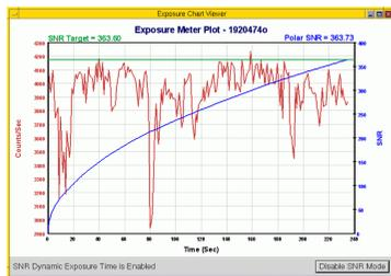
Observers can enable and disable the SNR mode (for programs that use the SNR mode). Using the Exposure Meter, they can follow at what rate the flux is coming (in red), see how stable the conditions are, and obtain a realtime measurement of the SNR (in blue).
