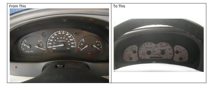
The original you can see the red, Theft light on the right side of the cluster between the oil pressure and battery indicators. The Theft light of the new set up is located on the bottom right corner of the speedometer.
