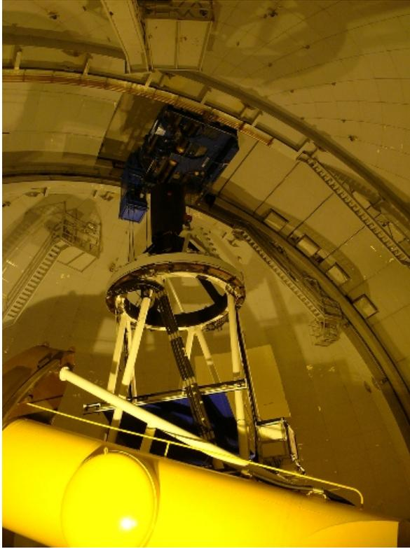
*WIRCam being mounted at the telescope with the upgraded upper end and prime focus cage.*
