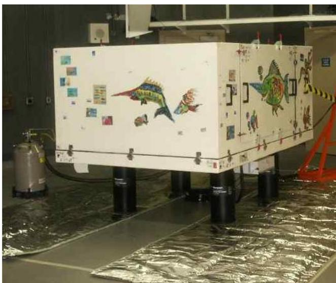
*The spectrograph in its thermal enclosure.*
