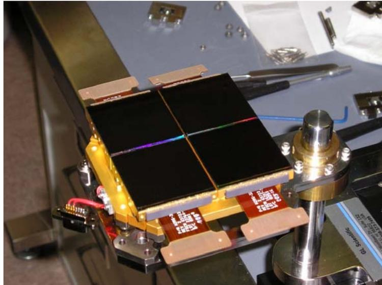
***The four science detectors are integrated at GL Scientific***
