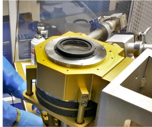
Figure 1: Installation of the SITELLE corrector lenses on the cryostats.
