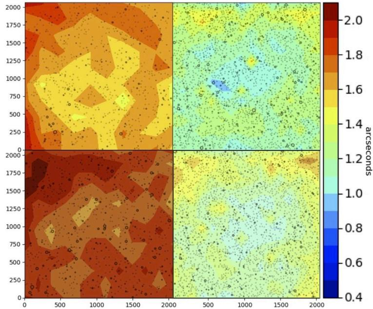
Figure 3: Comparison of the 90% encircled energy diameter (EED) before (left) and after (right) the installation of the focal plane correctors. Black circles represent stars used in the EED analysis.
