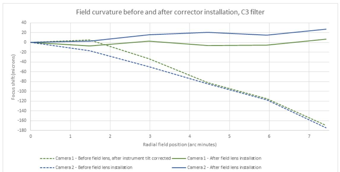
Figure 2: Best focus as a function of radial field position for SITELLE's cameras (Green and blue for camera 1 and 2 respectively). The dashed and solid curves respectively correspond to before and after the installation of the corrector lens for both detectors.
