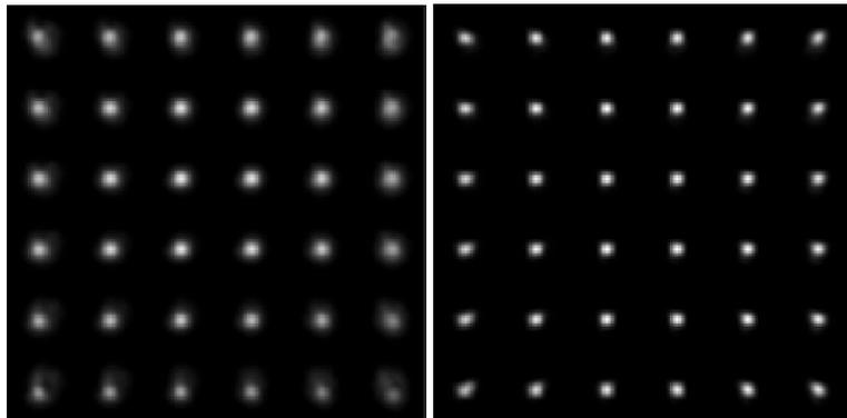
Figure 4: PSF of the stars in the SITELLE field of view before (left) and after (right) the upgrades. A linear grayscale intensity scaling has been applied.
