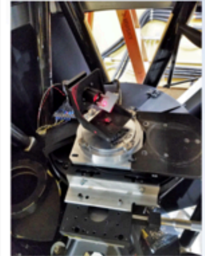
Above: The setup used to determine the alignment of SITELLE's collimator optical axis to the instrument mounting flange plane.
